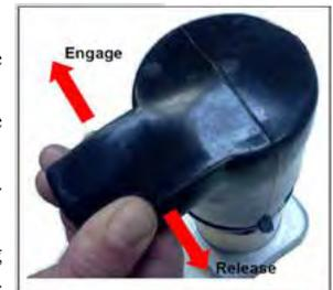
These parts are located inside the rubber boot wire tied over the motor. You must manipulate these parts **without** removing the rubber boot. **As noted on the side-by-side photo, removing this boot will void your motor warranty.** These photos will help you figure out how this works. The side-by-side photo (below) shows the spring lock lever and the brake lever.
