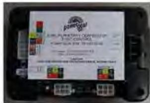
**Fig.1 Slideout Controller**
