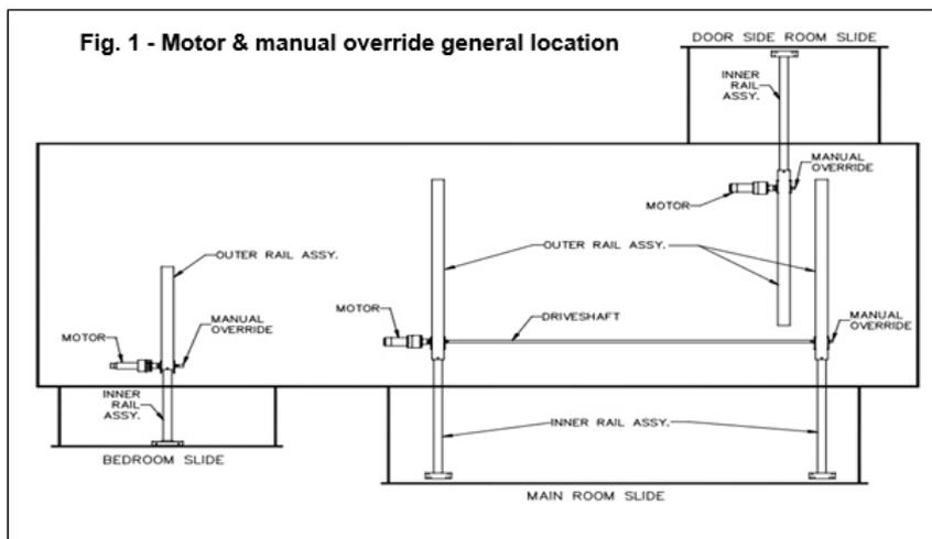
8. The room is now free to move. Using either a 5/8" or 3/4" wrench or socket, crank the room either in or out completely. If the slideout system is supplied with a gearbox override (optional), use the crank handle to move the room.
