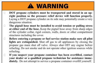
Propane "container" is a general all-inclusive term used to describe a vessel that is used for storage and delivery of propane gas.
