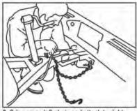
Criss-cross left chain and attach to right mounting slot in tow vehicle hitch.
