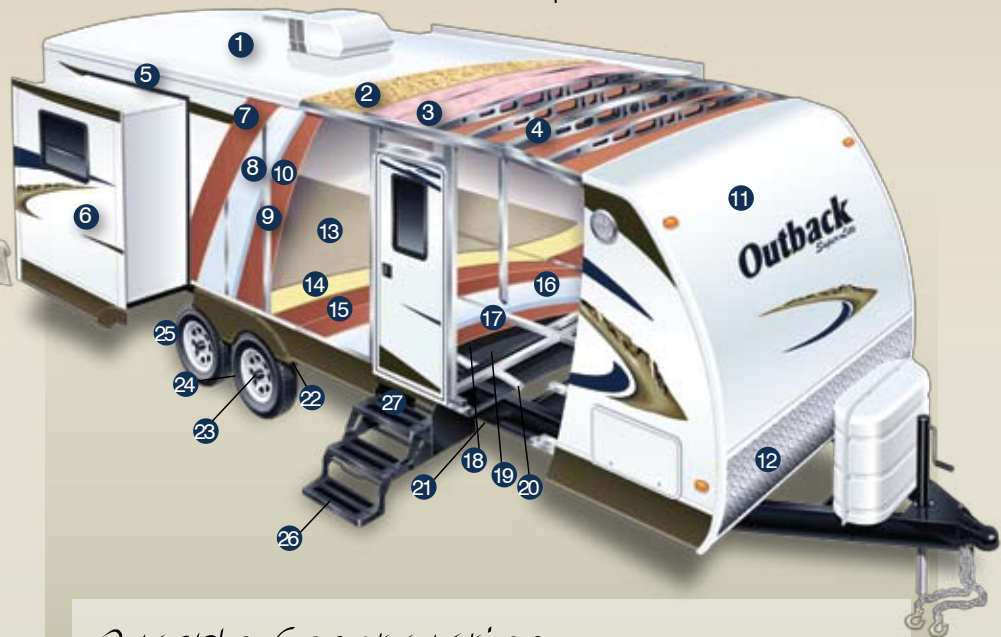
All Outback's are made with I-Beam chassis and full size outriggers. Pretreated in an 11 step process prior to painting ensures more rust resistance than our competitor's chassis.
