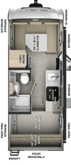
NEW! G19DBH LENGTH: 20' 8" WIDTH: 7' 8" HEIGHT: 10' 2" HITCH: 425 AXL: 2925 UWV: 3388 CCC: 1037 31 GAL 27 GAL 27 GAL
