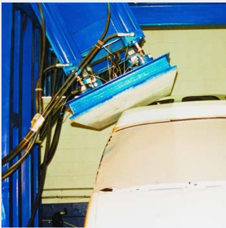
Roof crush resistance testing is intended to reduce deaths and injuries from roof crushing during rollover accidents.
