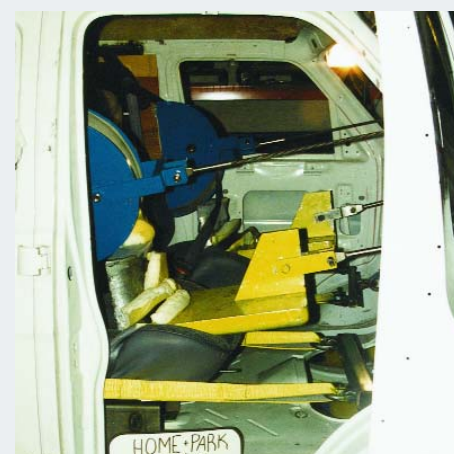
These 2 photos depict simultaneous seat belt pull testing and seating system testing. Seat belt testing confirms proper seat belt location and minimizes the possibility of anchorage failures. Seating system testing verifies the integrity of the seats, their attachments, mounting hardware and installation.
