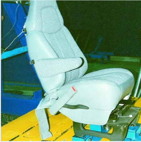
Seating system testing minimizes the possibility of failure of the seats, their attachments and their installation.
