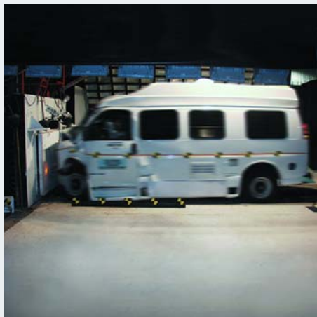
For frontal impact testing of the 190, the test vehicle impacted a fixed barrier at 30-mph (48 km/h). Again our test vehicle did not leak any fuel.
