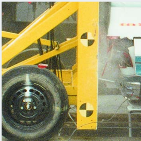
These 2 photos show the rear impact test on the 200 model. The test vehicle was impacted by a moving barrier at 30-mph (48 km/h). The entire fuel system was then inspected for leakage. Our test vehicle did not leak any fuel.
