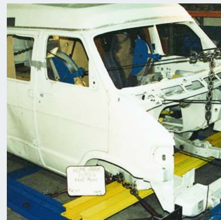
Occupant head protection testing is intended to ensure occupants have additional head protection from interior components during crashes.
