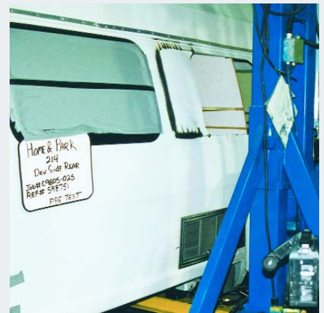
These photos depict side crush resistance testing which is intended to simulate the vehicle impacting a utility pole at a perpendicular angle.
