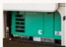
Standard ONAN 4.0kw gas generator gives you 30 AMP power when shoreline power is not available.
