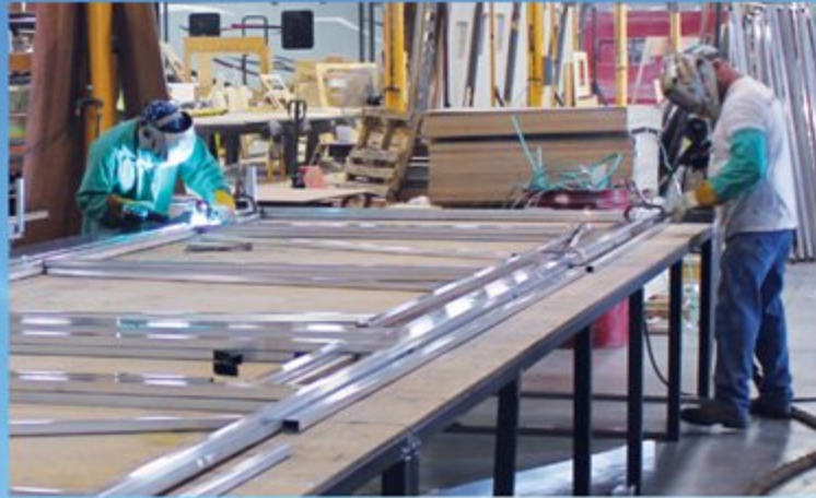
Micro Minnie features aluminum framing laminated with block foam insulation, true gel coat fiberglass exterior, and designer interior décor panels.
