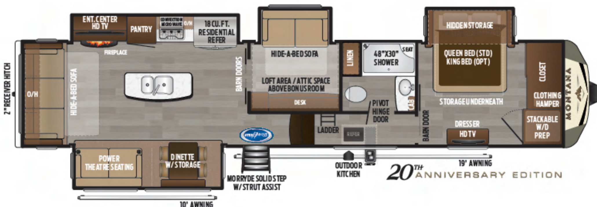
3854/3855BR Bonus room w/ loft and outside kitchen RV REFRIGERATOR RES. REFRIGERATOR Weight: 13630 LBS. | Length: 40' 10"
