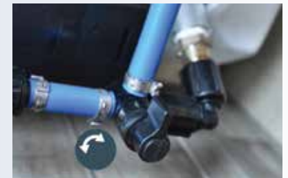
Water heater bypass & winterizing valves make draining the system for winter storage a breeze.
