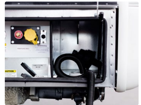
Macerator Sewage Discharge With Manual Disconnect
