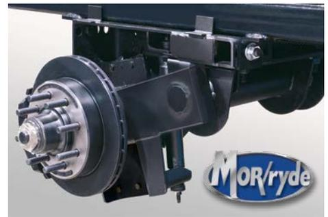
MORryde® I.S. Suspension eliminates the axle and leaf springs, allowing each tire to work independently. With 5 1/2" of travel per assembly, MORryde® I.S. will absorb road shock and protect your home for its lifetime.
