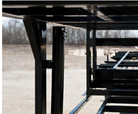
Pinless hydraulic jacks are mounted at a 5-degree angle for maximum stability.
