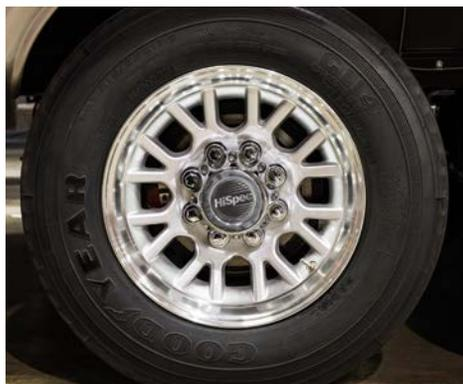
Heavy-duty 17.5" Goodyear® tires provide increased load capacity while staying cool on long hauls. We use truck tires, not RV tires, to ensure better performance and peace of mind.
