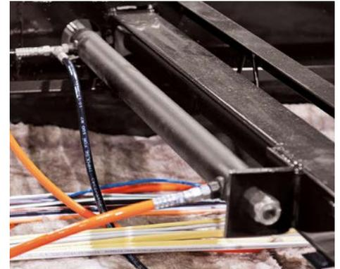
Commercial hydraulic rack & pinion slide-outs. All gear boxes are located inside the frame for the ultimate weather protection.
