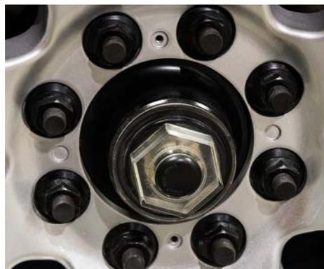
Commercial E-Z Lube® hubs surrounded by 8 large 5/8" stud bolts and standard automotive disc brakes round out the safety features of every DRV unit.
