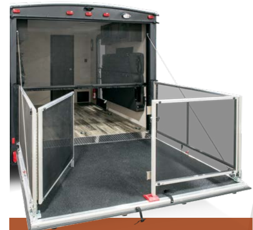
RETRACTABLE SCREEN WALL is optional, and pulls down like a garage door. And, host gatherings with the optional party patio package. (291THLE shown)
