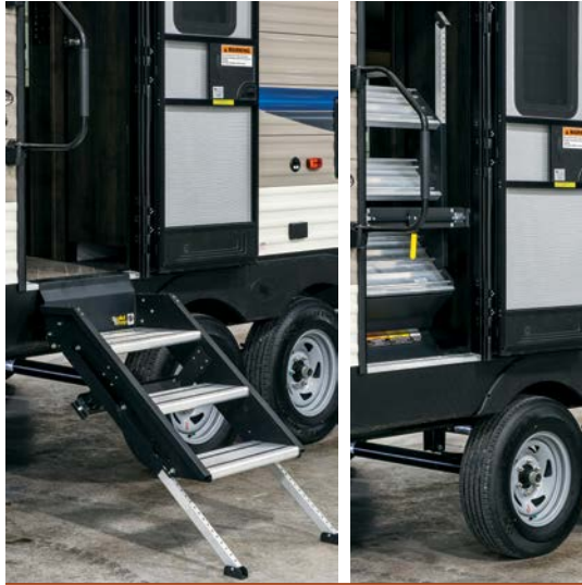
STANDARD FLIP-UP ENTRY STEP and friction-hinge entry door with folding grab handle. Step deploys squarely to provide solid footing, and flips up in one easy motion.
