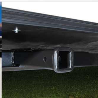
2" Accessory Receiver Hitch Every Avalanche comes standard with a 300 lb carrying capacity receiver hitch. Perfect for use with any accessory approved for RV use. Check accessory owner's manual.
