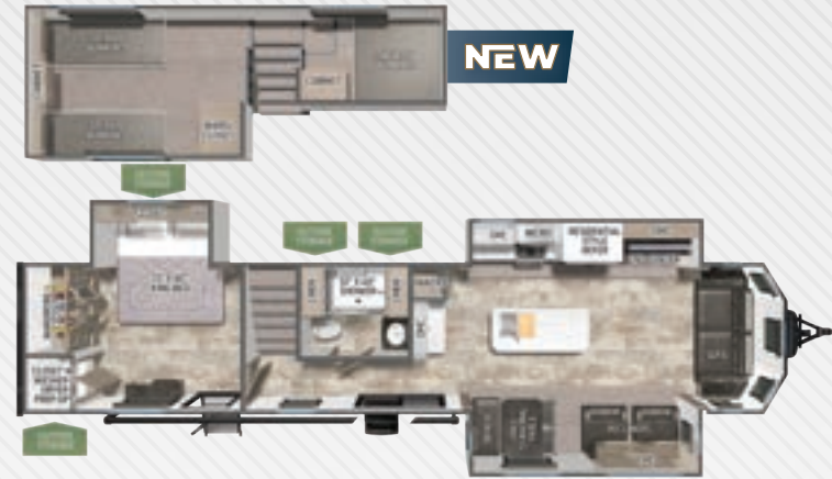
402FLT | LENGTH 42'10" HEIGHT 13'4" UVW 11849 HITCH 1695 AXLE 10095 CCC 2051 AWNING 21' 43 GAL 35 GAL 35 GAL
