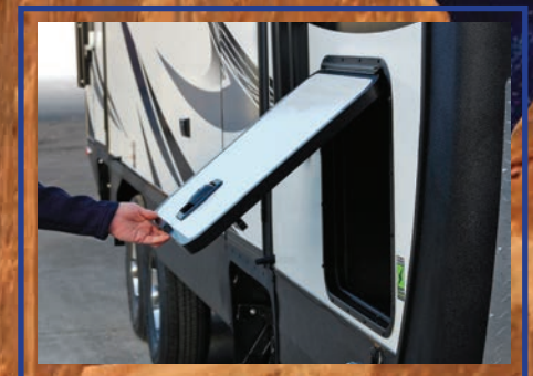
1" Thick Thermal Insulated Luggage Door Compartments
