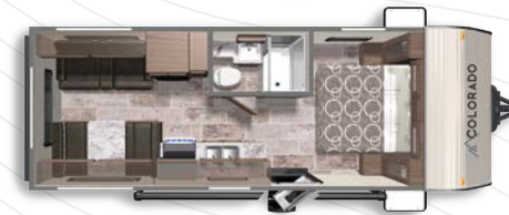
COLORADO 21RDC Length: 25' 5" Weight: 4,270 lbs. Sleeps: 4-6 Hitch: 528 lbs. Height: 11' 3"
