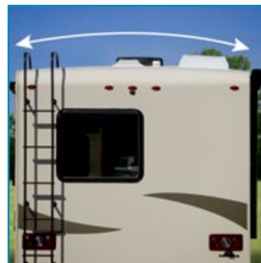
TPO Crowned Roof for Easy Water Runoff
