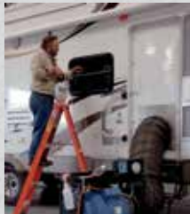
Seal Tech Air Pressure Test
