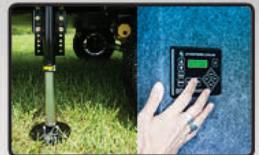
AUTO LEVELING SYSTEM
