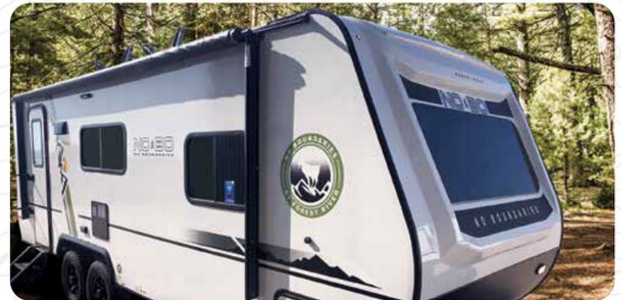
SEAMLESS PANORAMIC FRONT WINDOW 60" X 22" TEMPERED GLASS. FRONT CAP STANDARD WITH BACK COUNTRY PACKAGE ON 19 SERIES, OPTIONAL ON 16 SERIES
