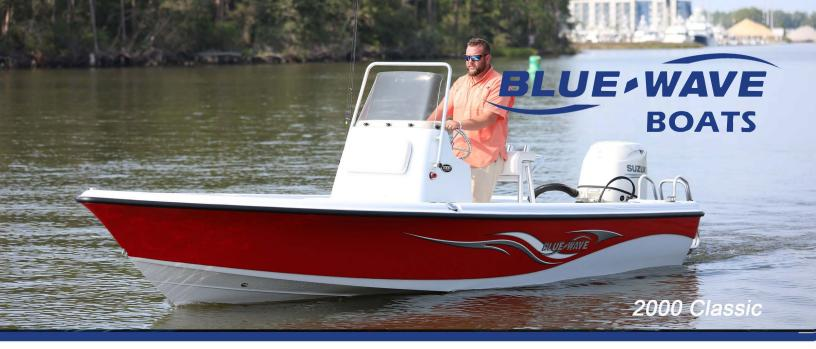
LOA: 20' 5" | BEAM: 8' | FUEL: 49 GALS | WEIGHT: 2,300 LBS | DRAFT: 11" | MAX HP: 150 Estimated Top Speed with Suzuki 140 HP: 44 MPH
