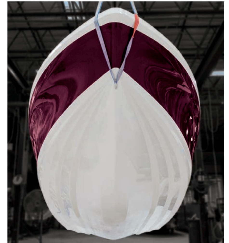
Perfectly prepared molds and careful gelcoat application create a mirror-like shine.
