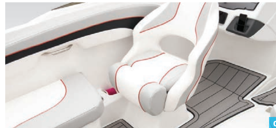
A. Water-resistant digital switches B. Bow anchor storage C. Flip-up helm seat bolster with swivel base
