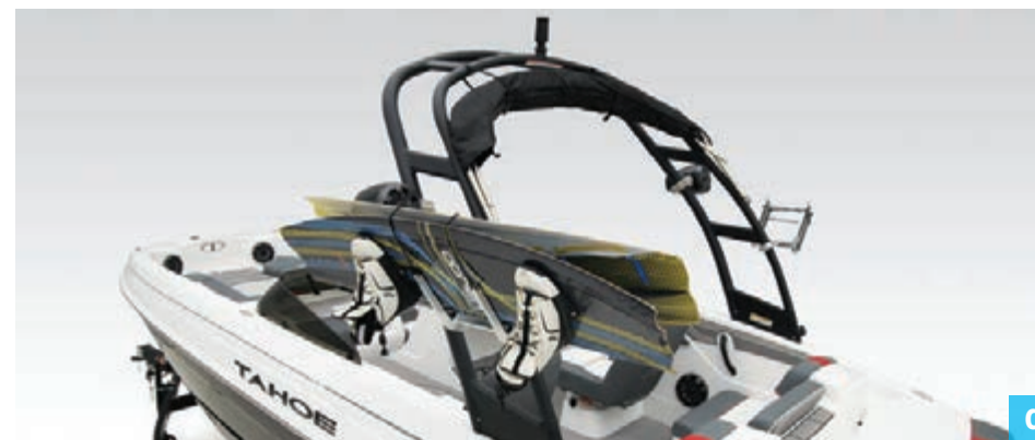
A. Cruise digital display & digital switches B. 3-across seating w/molded-in storage & flip-down seatback w/non-skid surface C. Optional folding wakeboard tower w/2 wakeboard racks, black bimini top & Optional KICKER® wakeboard tower speaker upgrade
