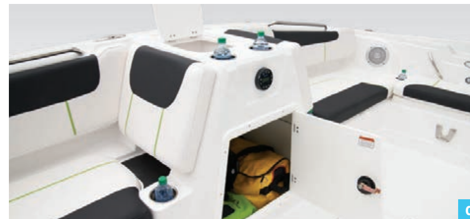
A. Flip-up helm seat bolster B. In-deck cockpit storage C. Port refreshment center w/storage
