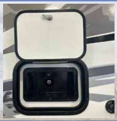
Exterior Pressure Washer/Portable Air Compressor
