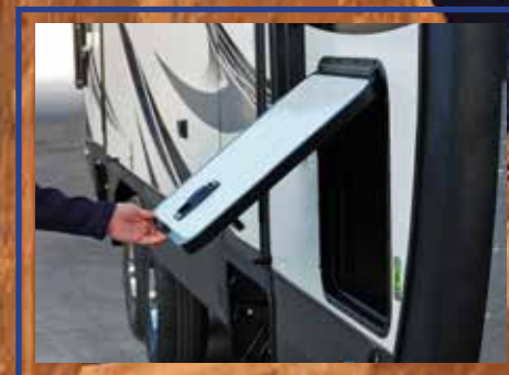
1" Thick Thermal Insulated Luggage Door Compartments
