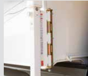
Swingout Jack Brackets - Allow for easy & secure loading & unloading. (Optional on 850, 960, 975 & 1062 / Standard 1172)
