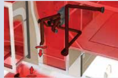
Ducted heat is routed into individually insulated holding tanks to keep them, the valves and PEX lines warm.
