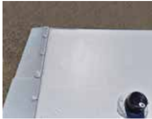
PVC Roof - The roof is covered in energy-star rated Polyvinyl Chloride (PVC) material. Integrated rain gutters and drip spouts prevent the sides of your trailer from streaking.
