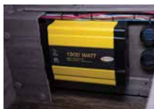
1500W Power Inverter converts battery power to 110V power allowing use of select appliances and devices including laptops, CPAP machines and others, while your away from shore power. (960 only)
