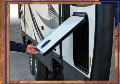
1" Thick Thermal Insulated Luggage Door Compartments
