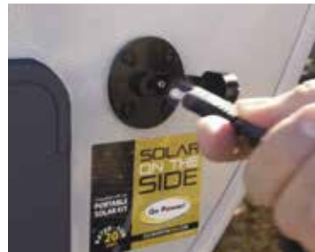
Standard Solar on the Side SAE port accepts external aftermarket solar panels to keep your 12v system charged.
