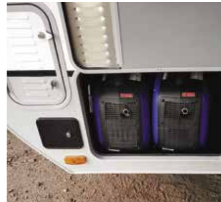
Portable generator storage compartment with tie down straps, accommodates Honda 2100 and similar sized portable generators. - N/A 1475, 1575 & 2465.
