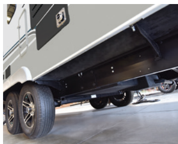
Standard HSLA e-coated frame protected against the mud, dirt and elements.
