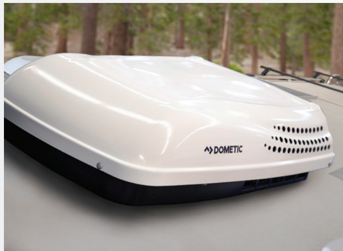
Dometic Penguin II 10K low profile a/c runs on 2,200w generator allowing for off the grid cooling.
