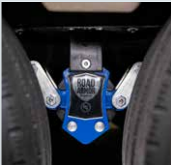
EXCLUSIVE Road Armor™ suspension Equalizes axle load to dampen shock and vibration
