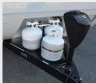
Tri-Five LP tanks allows extended off the grid use while an aerodynamic cover protects & conceals. - N/A 1475 & 1575
