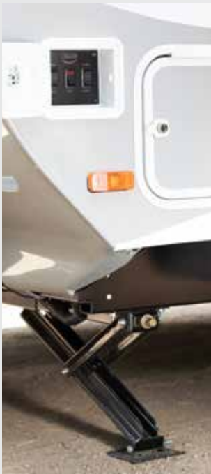
Electric stabilizer jacks with foot pads make set up & teardown sweat free, keeping your trailer rock solid while parked. - N/A 1475 & 1575
