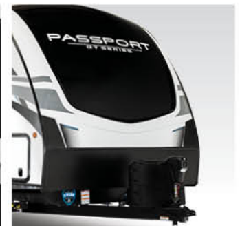
KEYSHIELD™ Automotive grade painted fiberglass front cap with chip and rock guard protection.
