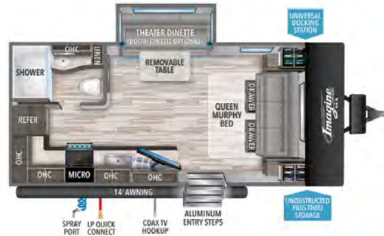
17MKE UVW' 4,674 HITCH' 480 LENGTH' 21' 11" HEIGHT 10' 5" CAPACITY 43 45 37
