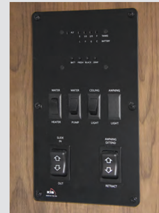
Standard Command Center Conveniently Controls Awning, Interior Lighting, Slide Out, Water Heater/ Pump, Battery Indicator Lights
