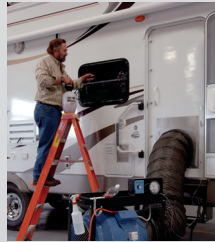
Seal Tech Air Pressure Test
