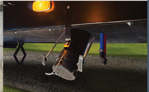
Termination Valve Service Light Standard on all models, this light allows adjustments to be made with two hands, no flashlight required.
