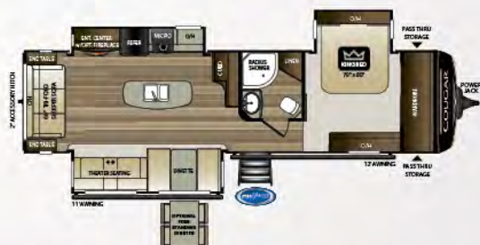
32RLI | Rear living room, three slides w/ bedroom slide Weight: 8801 LBS. | Length: 32' 10"
