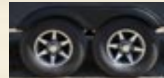
Optional aluminum wheels with Super Lube axles and ABS molded fender skirts
