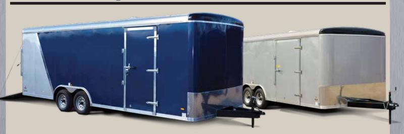
SUPERLOCK... Interlocking Exterior Aluminum system -unique to Haulin Trailers, lasts longer, looks much better, won't rust. The .030 interlocking aluminum panels are glued and mechanically fastened with fewer exposed screws.
