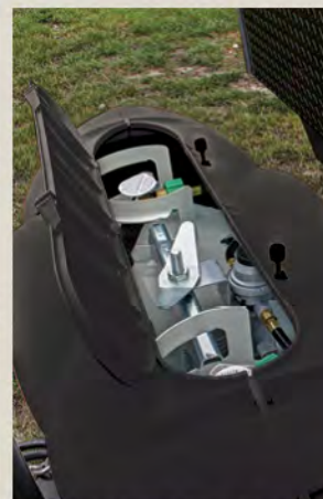
EASY OPEN LP TANK COVER W/DUAL TANKS
