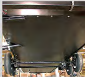
The Heated and Enclosed Underbelly
