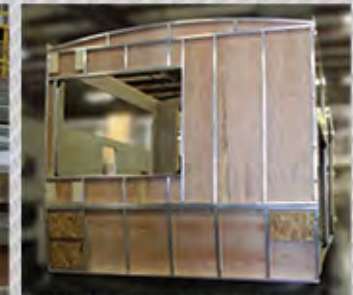
Double welded aluminum cage construction in walls and floors.
