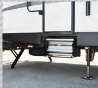
7.3 auto leveling system
