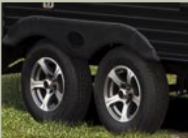
Tandem axles enhance stability
