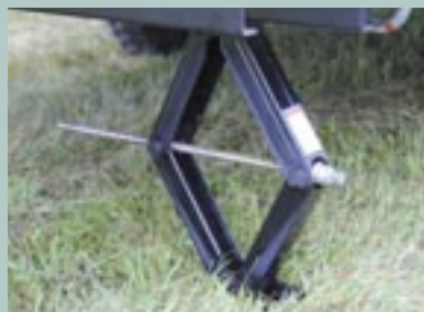
Four standard heavy duty stabilizing jacks
