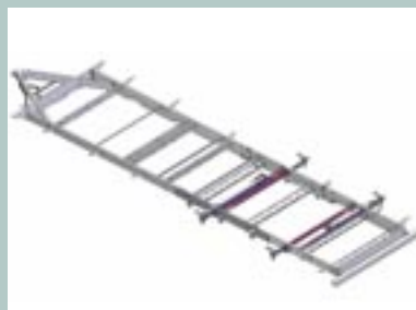
Norco NXG chassis featuring E-Coat technology
