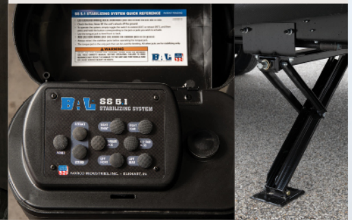
Norco™ Stabilization System (Premier only) Press OK and walk away! Electric jacks with large footpads and five points of contact quickly and consistently level and stabilize your RV.
