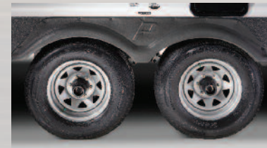
Grey steel wheel rims with Super Lube axles and ABS molded fender skirts
