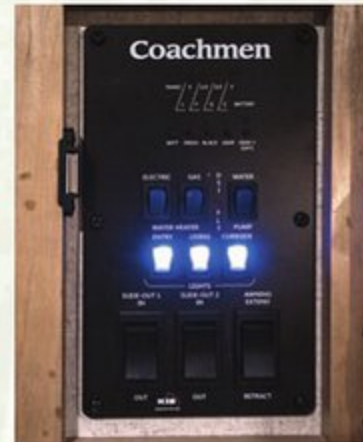
Centralized Control Panel indicates tanks, battery levels and operating components.
