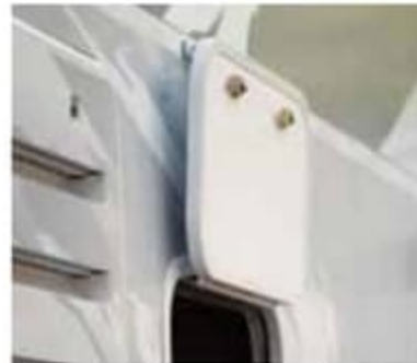
Magnetic exterior latches stay in place for hands free access.
