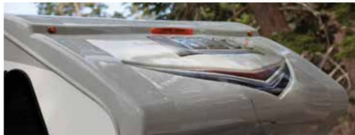
Aerodynamic TPO front nose cap protects your camper from debris and leaks while reducing drag and increasing fuel economy.
