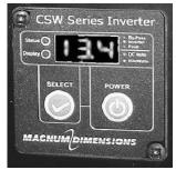
When in Bypass Mode you will be able to cycle through Battery Voltage, inverter settings and error codes. Inverter Power will not be available because the inverter is idle.
