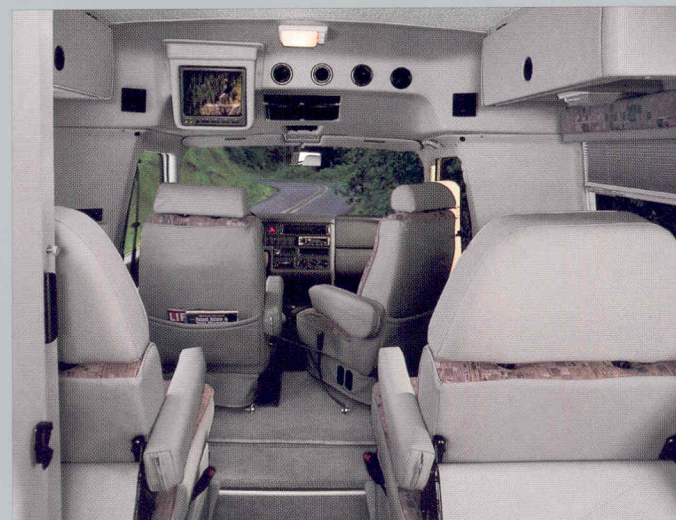
Cool comfort. Auxiliary automotive air conditioning located in the cab ceiling provides cooling for the coach area. A beverage tray with cupholders and storage bin is located conveniently between the driver and passenger.
