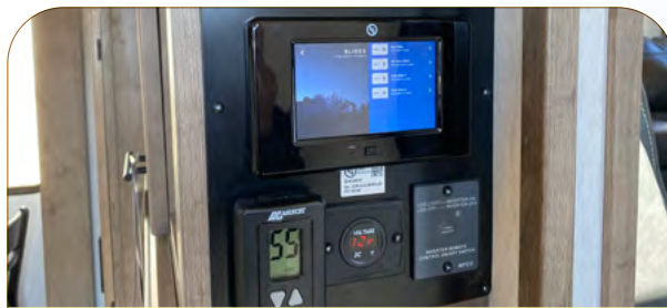
CENTRALIZED ONECONTROL SYSTEM FOR AUTO LEVELING, AWNING, SLIDEOUTS & LIGHTS WITH BLUETOOTH COMPATIBILITY
