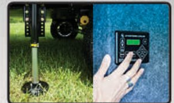
AUTO LEVELING SYSTEM
